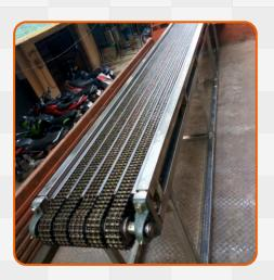
Chain conveyors are used to convey heavy unit loads, like pallets, grid boxes and industrial containers. Chain conveyors are single or double chain strand in arrangement. The load is placed on the chains; the friction of chains pulls the load.
