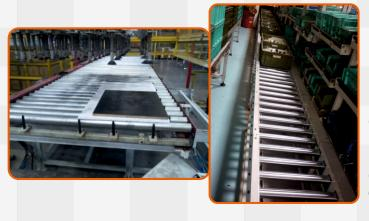
Motorized roller conveyor is manufactured in MS /SS round tube .the shaft with bearing at both ends with suitable load capacity is placed. The sprockets are in steel En-8 with hardened. Also sprockets are located in SS martial as per application Motorized roller conveyors are used to transfer boxes, bins, pallets. Gravity conveyors are used in transfer lines, logistics industry, ware houses, auto component handling, and food processing, dairy industry
