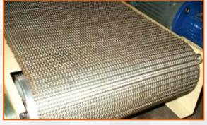
Cord weave belt is known within the industry as "Compound Balanced (CB)" belt. Compound balance weave has multiple spirals and cross roads per pitch. Which effectively creating a "belt within a belt". This compound structure closes up the spaces within the belt, it gives Compound balance weave its characteristic high density and flat surface.
